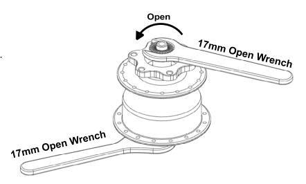
b) If the right side end cap (side with the plug) loosens first, you still need to take off the left end cap. After the right end cap comes off, use a 9mm wrench to anchor the axle on the right side, while using the 17mm wrench to loosen the end cap on the left side.
