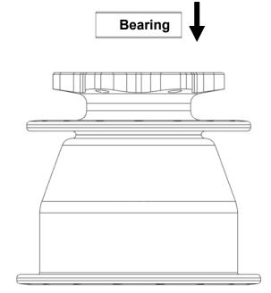
**STEP 6:** Install the old (or new) core assembly using a 30mm wrench
