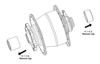
2. 36mm 板手旋開發電結構本體至空轉 Unscrew dynamo hub with 36mm wrench
